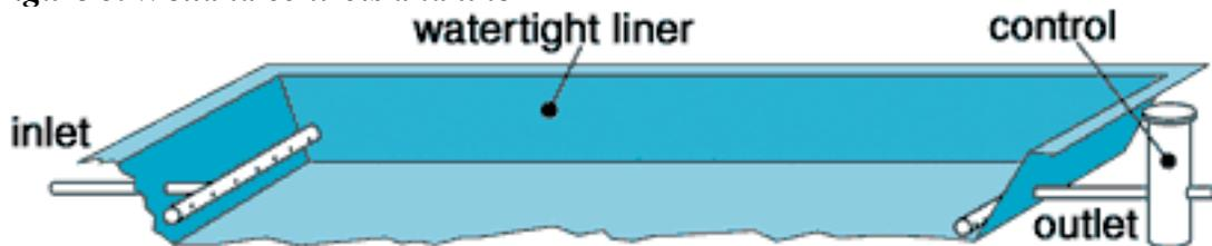
The *distribution medium* at the inlet is usually coarse drainfield rock that is 3/4 to 2 1/2 inches in diameter. This first part of the distribution system spreads the wastewater across the width of the wetland. Both gravity and pressure distribution can be used to spread the wastewater evenly over the system. The media in the filter is pea gravel that is 3/8 to 3/4 inch in diameter. The depth of the pea gravel varies from 18 to 24 inches.
