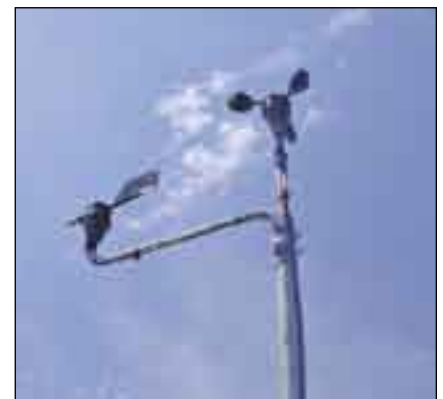
An anemometer (right) and a wind vane (left) measure wind speed and direction.
