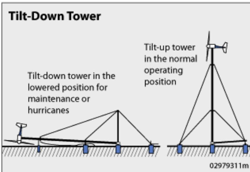
Guyed towers are easier to install than self-supporting towers. However, because the guy radius must be one-half to three-quarters of the tower height, guyed towers require enough space to accommodate them.
