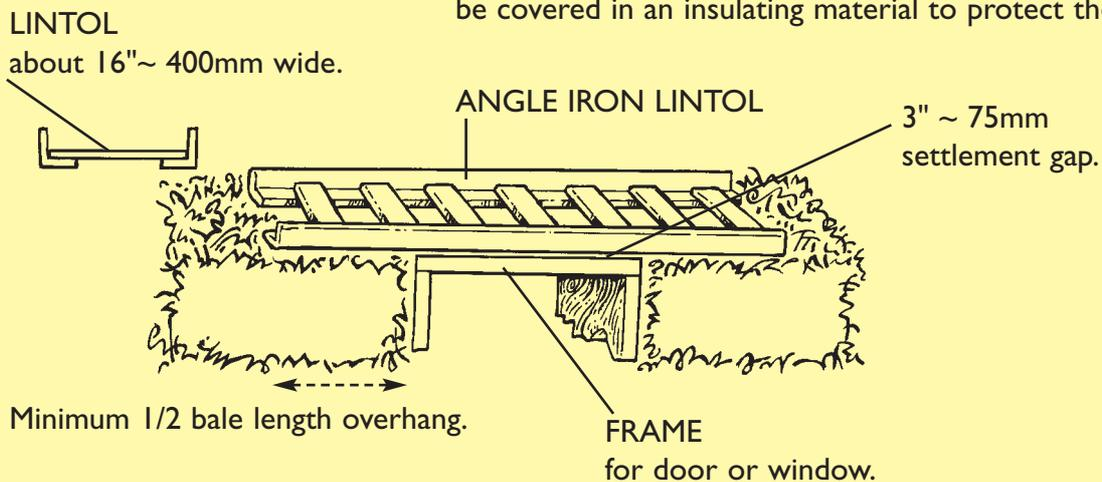
2. **ATTACH** the window and door box frames directly to the wallplate above it. This can be a good option if the design calls for tall windows, but a settlement gap must be left **below** window frames in this case. It has the advantage of reducing the amount of timber required for the frame. However, it is probably only a first choice option on the ground floor of a 2-storey house, as otherwise the overhang of the roof would obscure much of the light.
